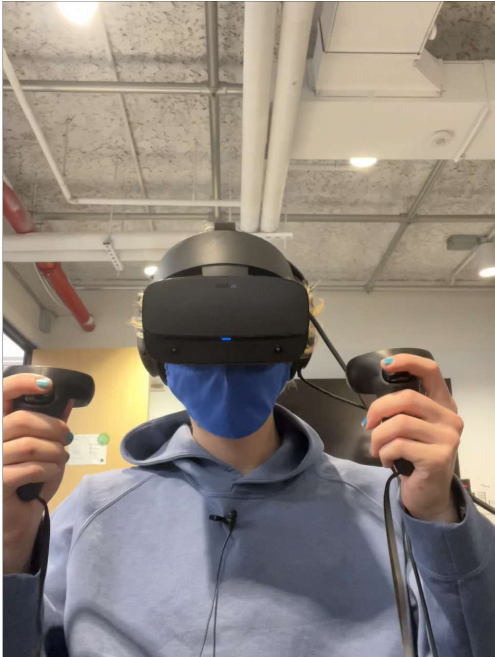
Figures 16 (Top) and 17 (Bottom) Depicting Users Wearing VR Headset, Controllers, and Headphones with a Shure SM58 and a Sennheiser ME 2 Lavalier Mic
